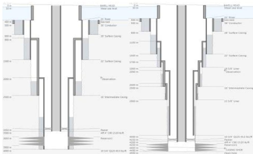
In addition to this, a packer inside the open hole is drawn from the tubing to the outer edge of the open hole. This was not drawn in previous versions.
